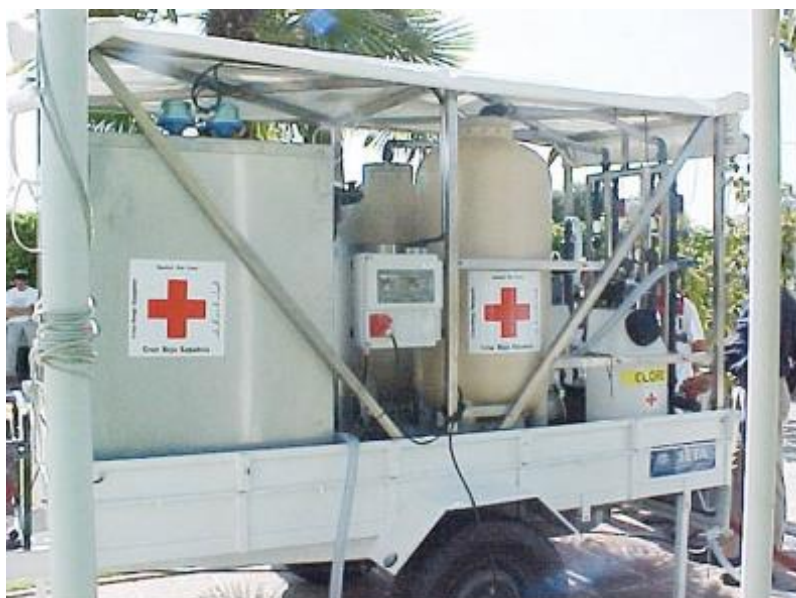
Trailer-mounted water treatment unit (IFRC SETA unit – capacity 3000litres/hour) this set up also has activated carbon filters to remove any odors
